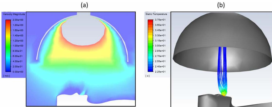
Figure 2: Preliminary CFD results of AIIED. (a) velocity distribution; (b) pathline of airflow representing breathing.
