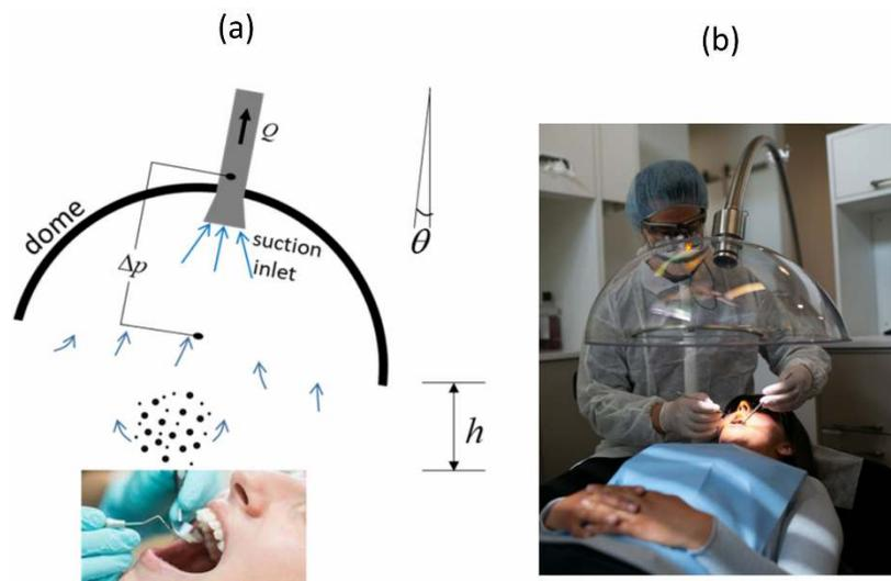
Figure 1: (a) Working principle of AIIED; (b) Application of AIIED.
